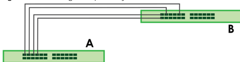
Figure 114 Trunking Example – Physical Connections
