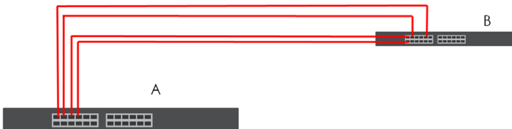
Figure 112 Trunking Example – Physical Connections
