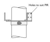
Mounting positions for Mounting bracket up to 5 No. PIR's adjustable on pivot bolt
