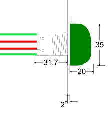
If used externally silicon sealant MUST be applied around the faceplate and fixing holes to achieve IP67 rating.
