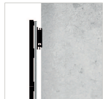
Close to the wall install - Only 124mm from the wall to the front of the panel
