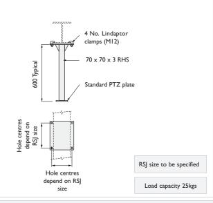
All brackets for camera mounting have a Ø127 mounting plate with Ø8.5 holes equi - spaced on 101.6 PCD
