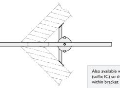
Also available with internal cable way (suffix IC) so that cabling is concealed within bracket
