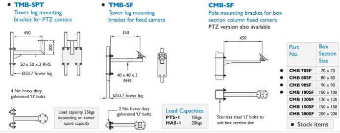
All brackets for camera mounting have a Ø127 mounting plate with Ø8.5 holes equi - spaced on 101.6 PCD
