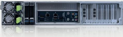
The rear view of VIEWSPAN Plus 6 shows the mirrored, solid-state, 2.5" removable OS drives and the dual hot-swap PSUs. The six screen outputs are in two rows on the right. Only the two RJ45 network connectors on the main panel are used (1 x Gb, 1 x 10Gb Ethernet)
